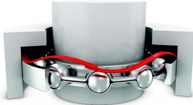
The SSB series is a popular choice among engineers, the single turn wave spring helps eliminate bearing play and minimize noise. The constant light/medium pressure they apply removes play between the ball bearings and the bearings' inner and outer races. Preloading can reduce the possibility of bearing damage due to vibration (vibratory loading) and wear due to repetitive and non-repetitive runout.
