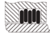
YSK Series QSK Series External - Medium Duty 1 set = 5 individual rings (3 rings rotate with shaft & 2 rings rotate with bore)
