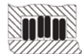
YSKD Series QSKD Series External - Heavy Duty 1 set = 3 individual rings (2 rings rotate with shaft & 1 ring rotates with bore)
