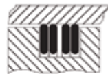
YHD Series QHD Series Internal - Medium/Heavy Duty 1 set = 2 individual rings (rings rotate with bore only)
