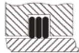
YS Series QS Series External - Light Duty 1 set = 3 individual rings (rings rotate with shaft only)
